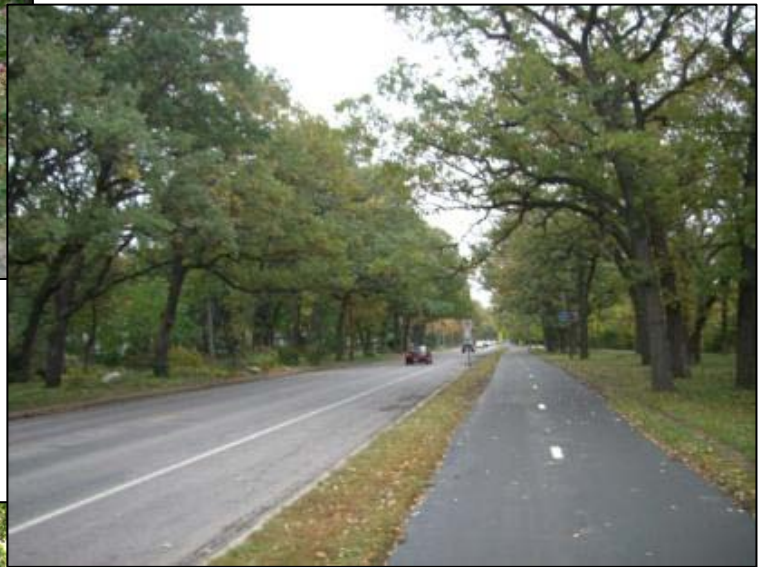
A multiuse trail (sidepath) is located within or near a road right-of-way and provides separation from traffic
